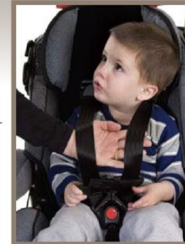
Adjust harnesses so both sides are the same length
